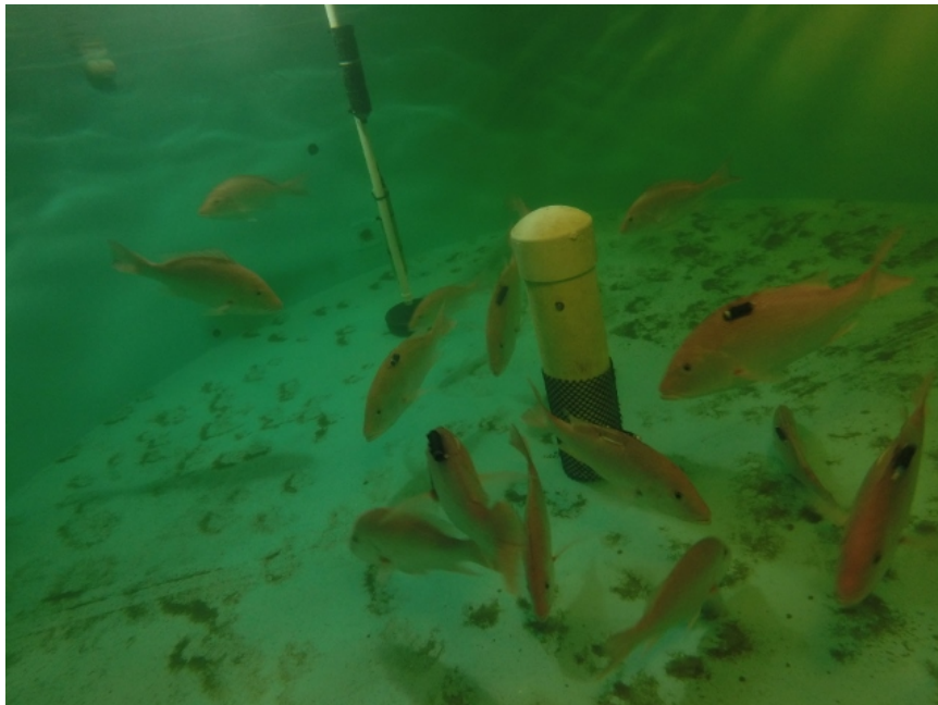
Figure 1. Hatchery tank where preliminary tagging trials occurred. A subset of Red Snapper were tagged with a variety of transmitters of varying size and specifications. Acoustic receivers (seen towards back of tank) recorded acoustic detections from the tagged fish and transmitters fixed to stationary poles.
