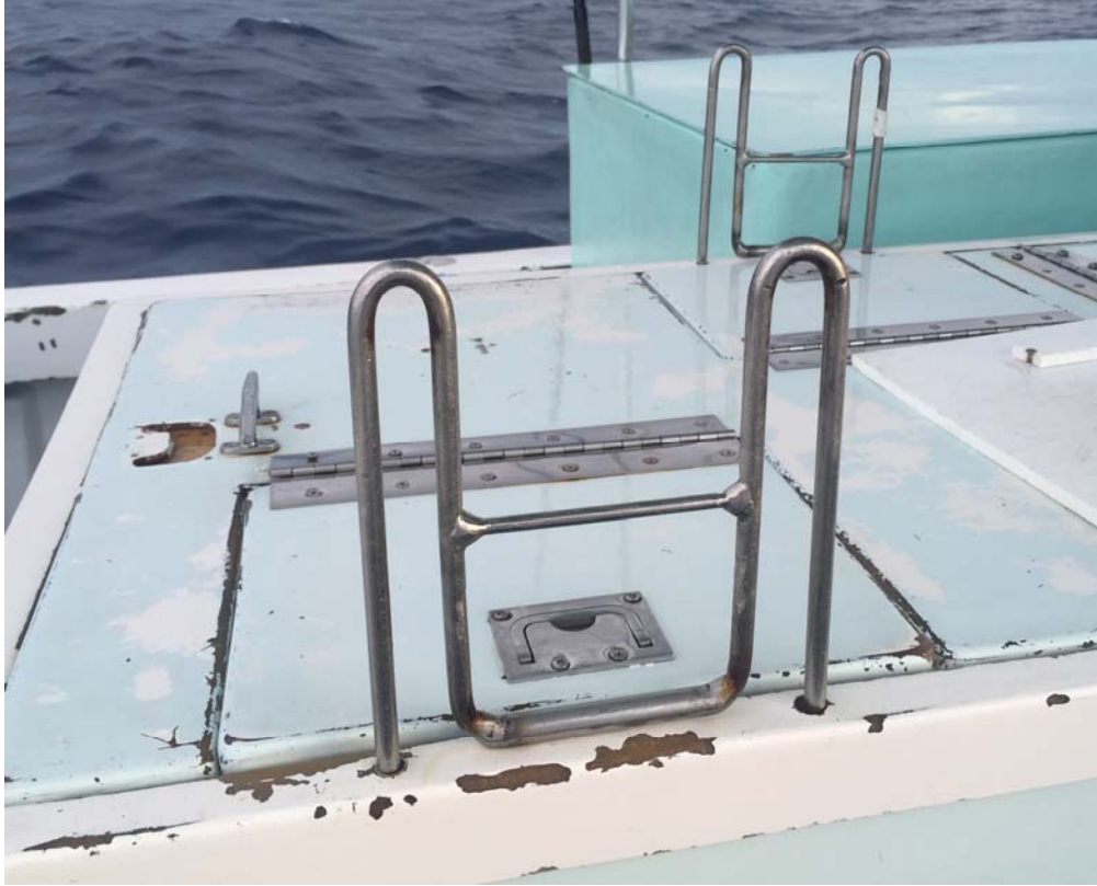
Figure 3.1.1. An example of a purpose-built yellowtail snapper dehooking rig from a commercial yellowtail snapper vessel. The fish is lowered into the fish box, and the fishing line is then pulled over the crossbar. The hook catches on the crossbar, dehooking the fish, which then falls down into the fish box.
